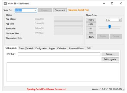
If application can't open the Serial Port, check device manager to confirm the correct serial port number is selected.
