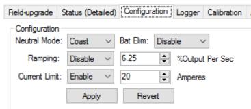
Brake vs Coast in neutral can be selected in the configuration tab. Additionally, the battery eliminator can be enabled here.
