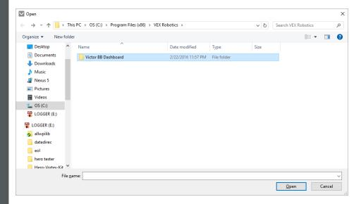
Navigate into Program Files (x86)\VEX Robotics\Victor BB Dashboard\Firmware files
