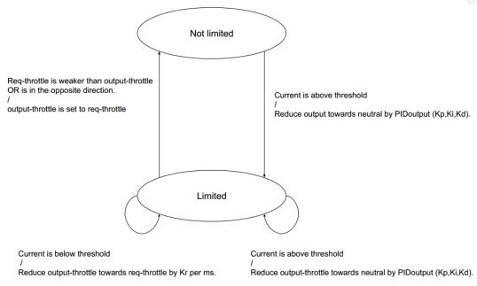
D-gain can be used to hasten the response as a function of the rate of change of the current-error.
