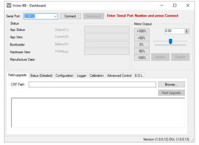
Bring down the dropdown and select the appropriate COM port. If the list is empty, then no serial cable is attached to the PC or drivers are missing. See Section 2.1 for instructions.
