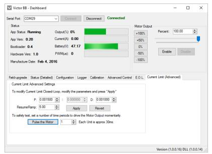
The additional advanced tab allows customization of the P-gain, D-gain, and Resume rate (Kr).
