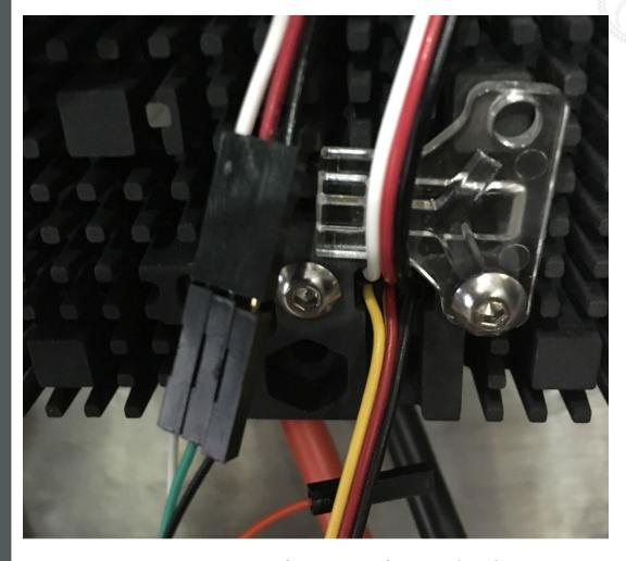
You can directly connect the Adafruit UART-USB cable (Adafruit product ID: 954) to a standard PWM cable as shown above.
