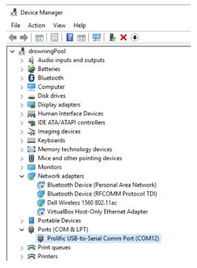
At this point you can insert a Serial USB Cable and it will appear in device manager.
